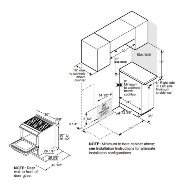
Provide adequate clearances between the range and adjacent combustible surfaces. These dimensions must be met for safe use of your range.
