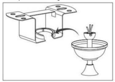
After wiring ,attach the canopy to the hanger bracket by pushing up and twisting to locate screws in key holes then
