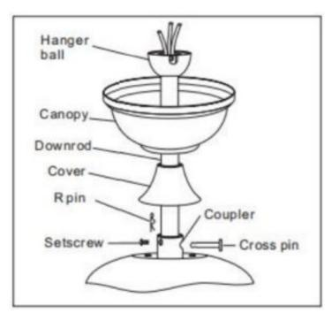
Carefully lift fan assembly into hanger bracket that is just attached to the outlet box. Be sure the groove in the ball is lined up with tab on the hanger bracket.
