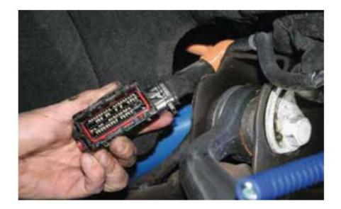
**Step 3**Route switch through firewall. Locate pin 11 & 35 & push out the plastic plugs from the top side down. 2011 Duramax's will sometimes have a yellow wire in pin 11, that wire is okay to remove or piggyback off of the SOTF wire.
