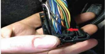
**Step 5**Reinstall top cover and bottom retainer. Use a zip tie to secure the loom from your switch to the ECM harness.
