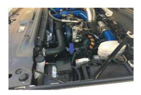
Route connector through the wheel-well, remove the plastic top cover and pin retainer.
