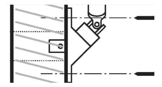
6. Insert the tube (cut to length) and fix the plate to the wall (fixings not supplied).
