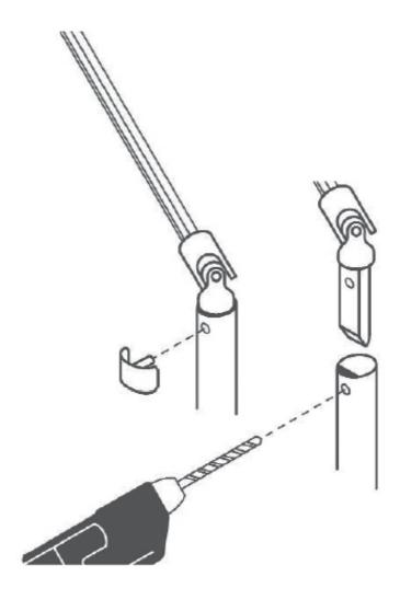
4a. Option 1 – installing the lock tube to the side of the guide rail
