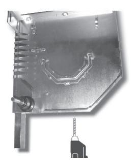
2. Remove the screw from the end of the hexagonal bar. Insert the bar through the override hole then secure in place using the screw. This is to prevent the handle from being pulled out during use. (3mm Allen key)
