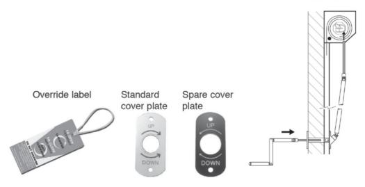
Internal and external operation Low Level Override Kit
