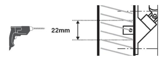
4b. Option 2 – Installing the lock tube through a face fixed guide rail
