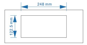
2. Place the product into the opened square hole, press it tightly, and fix it with screws, as shown below:
