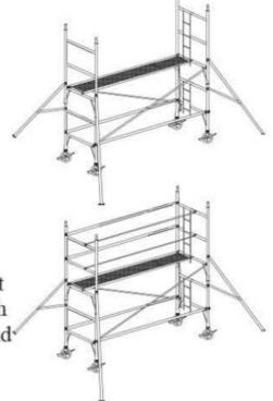
8: Using the 3T method of assembly, fit horizontal bracing on the 4th and 5th rungs. The platform is now safe Stands On.
