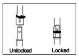
2. Snap pins - Unlock the interlock Clips on all frames. When installed, always move the interlock clip to the
