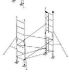
7: Place platform on the 5th rung ensuring hatch is to the ladder end and it opens outwards, check the platform is secure and level then lock the windlocks. Using the 3T method of assembly, fit horizontal bracing on the 6th and 7th rungs, the platform is now safe to stand on. Please note you need to use a Platform on the 1st Rung
