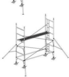
9: Using the 3T method of assembly, fit horizontal bracing on the 5th and 6th rungs. The platform is now safe Stand On.
