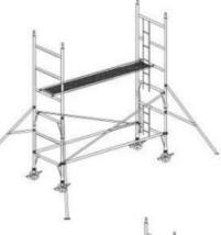
5: Fit 2 diagonal braces in opposing direction from the 3rd rung to the 5th rung as shown
