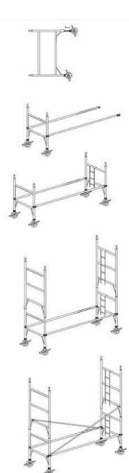
6: Place platform on the 3rd rung ensuring hatch is to the ladder side and it opens outwards.check the platform is secure and level then lock the wind locks.
