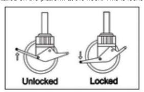
4. Wheel lock – Install castor/leg assembly to frame by pushing the leg into the frame tube. This Should be done with manual force only, no tools. Lock Castors before ascending any part of the tower.
