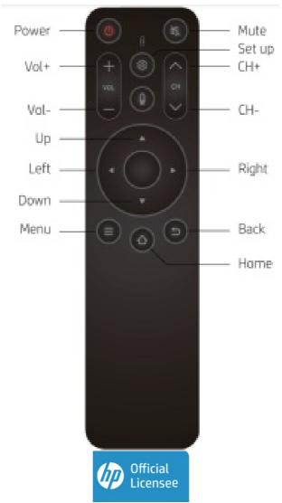
The product sends out a Bluetooth remote control pairing request. Press the menu and return button for more than 3 seconds to complete the remote control pairing, and then the Bluetooth remote control can be used normally. **Key Description: Power:** Turn on/off the product
