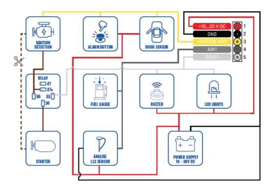
This diagram outlines an advanced wiring circuit to utilise all features of the tracker, for a basic installation you will only need to connect Battery, Ignition and Ground.
