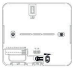
5. If powered by conductors external to the wall, fix the conductors with the cable clamp supplied and protect them in a suitable electrical duct.
