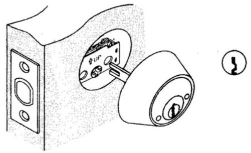
C. Insert(2) two screws through countersunk holes engaging holes in exterior cylinder and tighten.
