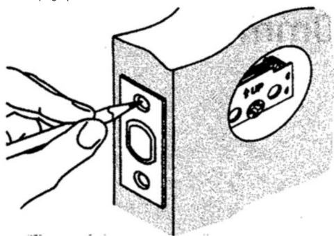
B. Chisel 1/8" deep or until latch face is flush with door edge.
