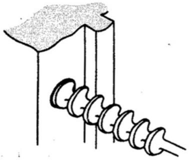
B. Mortise 1/16" deep for strike locating from 1" hole in door insert and tighten screws.
