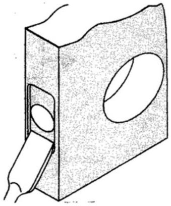
C. Install deadbolt latch in up position into hole as shown latch insert and tighten screws.
