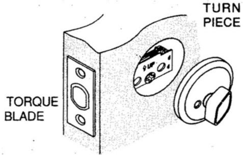
B. Insert machine screws through holes engaging holes in cylinder and tighten.
