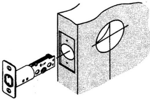
D. For round face deadbolt press flush to door edge Bolt must for be vertically aligned with door edge as indicated by arrow.
