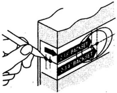
B. Mark center hole on door face through guide on template for either 2-3/8" (60mm) or 2-3/4" (70mm) backset.
