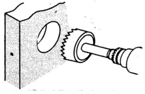
B. Drill 1°(25mm) hole in center of door edge thru to 2"(50.8mm) hole for latch.
