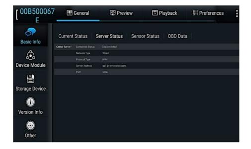
If the device is connected to the server, the status will change to 'Connected'. To check the sensor status, navigate to General>Basic Info>Sensor Status.
