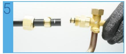
6. Insert the nipple of the fitting into the end of the pipe making sure that the pipe fully seats into the bottom pocket of the fitting adaptor and the mark is at the thread of the adaptor.
