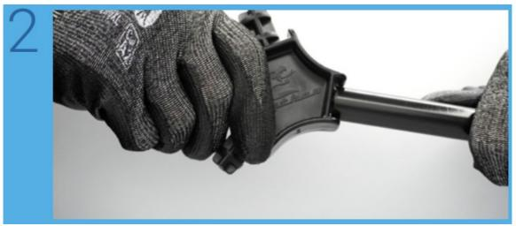
3. Mark the pipe, at the reference shoulder of the chamfer tool, before removing the tool and be sure the pipe chamfered debris is pulled away from the end of the pipe.
