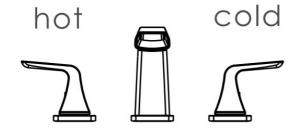
2. Contrarotate the left handle i for hot water the greater angle you open, the larger flowrate you get. Conversely the smaller angle you open, the little flowrate you get fill turn off. Clockwise rotation the right handle is for cold water, the greater angle you open, the larger flowrate close close you get. Conversely the smaller angle you open, the little flowrate you get till turn off.
