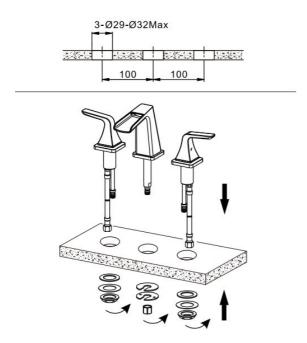
2. Use hand fo screw up the lock nut, then use install tool for fixing strengthen. And then connect the outlet hose as shown.
