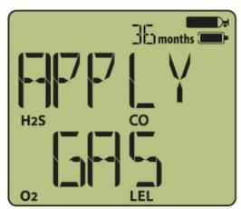
**Warning** – DO NOT auto-zero the detector in a combustible atmosphere.
