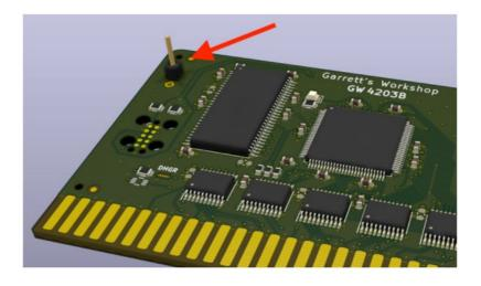
For customers purchasing a new RAM2E, we can at your request mount a special connector that supplies a buffered copy of the 14.318 MHz clock signal. Connect the VGA Scaler's 14 MHz clock wire to this header. A picture indicating the location of the 14 MHz clock header is shown to the right.
