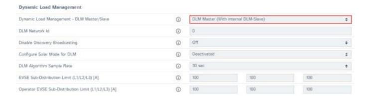
2. Set EVSE Sub-Distribution Limit and EVSE Sub- Distribution Limit to groups fuse value
