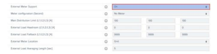
5. Choose the correct meter type according to the installed external meter on the dropdown menu for "Meter configuration (Second) and set "Main Distribution Limit" to the fuse value where the external meter is located and measures
