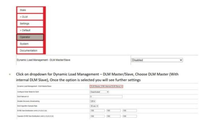
2. Set **EVSE Sub-Distribution Limit** and **EVSE Sub- Distribution Limit** to the ampere that's always available to the group of chargers.
