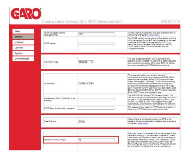
3. On bottom of the screen, click "Save & Restart" to save the configuration. Once the controller has been restarted the operator current limit should be set, and you can now try a charging session to confirm.
