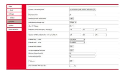
DLM Network ID – should be changed to a number for the rest of the chargers to find it. We recommend using "1". EVSE Sub-Distribution Limit – This is where you set what AMPS are always available to the group of chargers. Always set the values of "EVSE Sub-Distribution Limit" and "Operator EVSE Sub-Distribution Limit" to the same value during setup.
