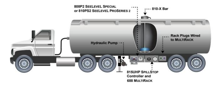
The SPILLSTOP controller works in conjunction with alarm signals sent by the 808P2 or 810PS2 level gauges and hose pressure sensors.
