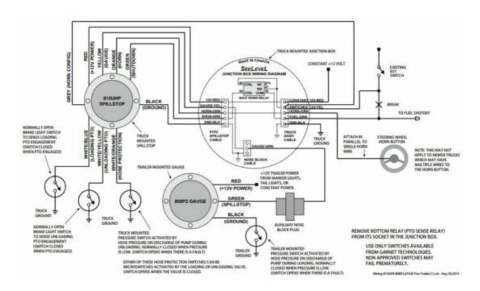
WIRING DIAGRAM – ONE COMPARTMENT WITH 808P2 GAUGE, 815UHP SPILLSTOP AND 815JB JUNCTION BOX TRACTOR TRAILER APPLICATION, TRACTOR MOUNTED UHP & JB, BOTH HOSE PROTECTION SWITCHES ON TRACTOR.
