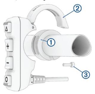
2. Place the handlebar controller mounting clamp 2 over the bushing, making sure the ridges on the bushing match up with the grooves in the mounting clamp. match up with the grooves in the mounting clamp3.
