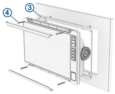
On ECHOMAP UHD2 9 sv models, the top and bottom gasket pieces are not interchangeable and are labeled to help install correctly. Be sure to use the appropriate gasket pieces on the top and bottom to avoid water ingress behind the mounting surface.
