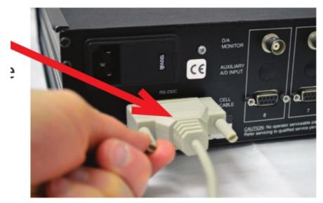
4. Attach the Potentiostat/ECM8 cable to the cell cable jack on your potentiostat. Attach the other end of the ECM8 cable to the multiplexer POTENTIOSTAT receptacle.
