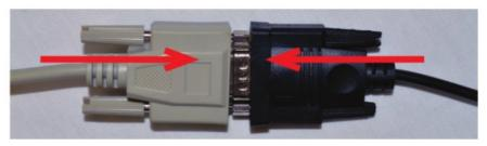
2. Plug the USB-to-serial converter cable into a free USB port on the host computer. Windows® detects the cable and assigns a COM port number.
