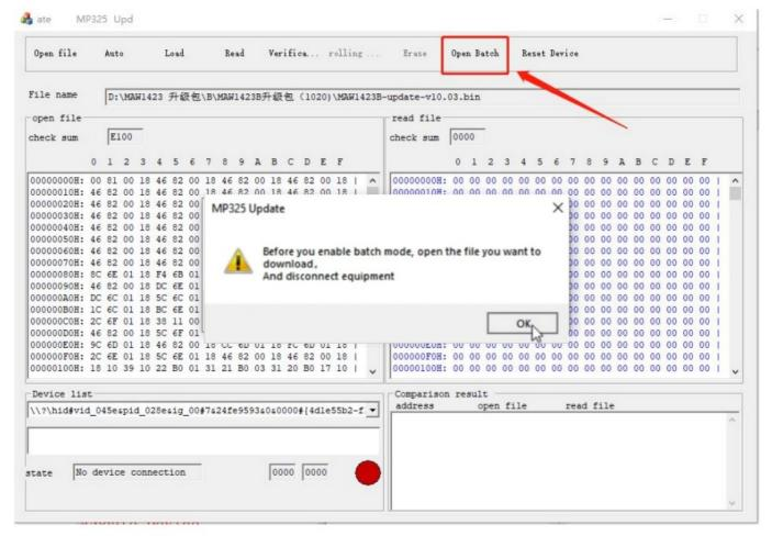
9.The controller holds down the UP button and connects the controller computer with a data cable. The controller indicator light flashes – the tool automatically upgrades the device. After running the progress bar, the upgrade is completed
