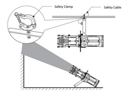
Never stand directly below the device when mounting, removing, or servicing the fixture.
