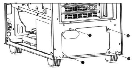
Lock 4pcs psu screws to fix psu
