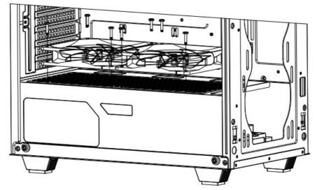
Put fan on upside of psu cover and fix screwss
