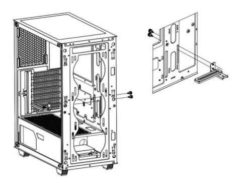
Put VGA card on M/B and fix 2pcs screws. available to adjust the height of VGA card
