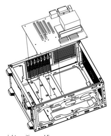
Put M/B to chassis on right position and fix screws
