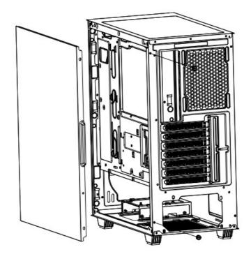
Put side panel on right position and push it, then lock 2pcs screws
