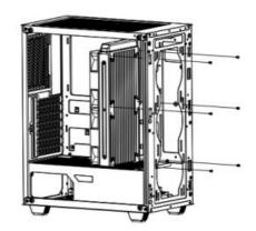
Put fan or water cooling on front plate from inner side and fix screws from outside
