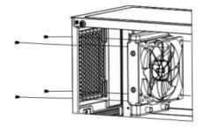
Put fan or water cooling on rear plate from inner side and fix screws from outside
