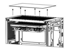
Put fan or water cooling on top panel from inner side and fix screws from outside
