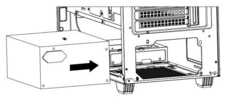
Put psu into chassis from left side
