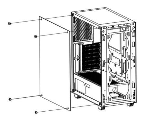
Put side panel on right position and lock 4pcs screws
