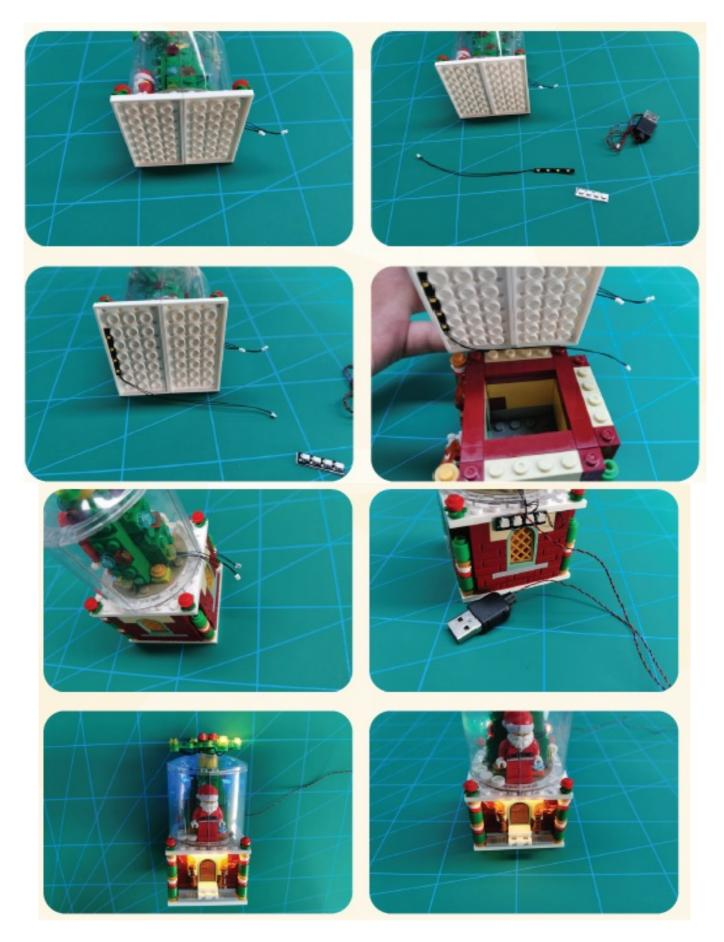
Connect the light kit to the battery box and installation will be complete. If you would like to use another power source, please make sure the maximum voltage is 6V.
