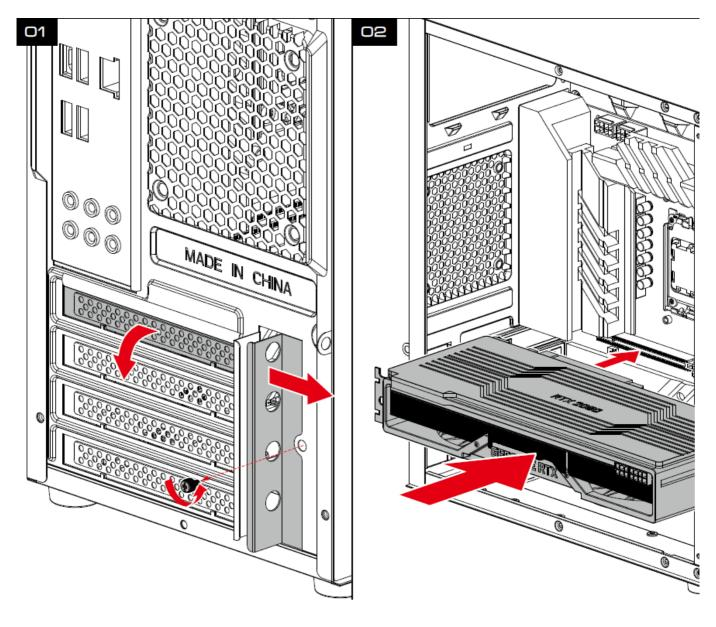
Identify the PCI-E x16 slot on the motherboard, usually the largest slot, closest to the CPU. Align the graphics card's connector with the PCI-E slot and gently press down until the card is firmly seated in the slot.
