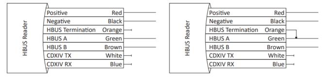
**Note:** To terminate an HBUS Reader, connect the **Orange** (HBUS Termination) wire to the **Green** (HBUS A) wire.Cardax IV Reader connection:
