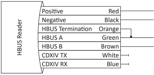
Note: To terminate an HBUS Reader, connect the Orange (HBUS Termination) wire to the Green (HBUS A) wire
