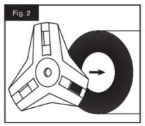
2. Install Film Roll: Slot the narrow side of the film clamp into the roll of film. Make sure that the large side of the film clamp is flush with the roll (Fig. 2).
