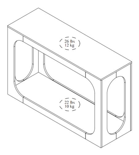
This unit has been designed to support the maximum loads shown. Exceeding these load limits could cause sagging, instability, product collapse, and/or serious injury.
