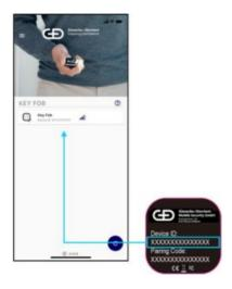
8. Enter the pairing code printed on the reverse side of the StarSign Key Fob in the connection menu. The check marks in the dialog can be ignored.
