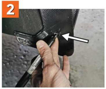
A. Rotate the mud guard to align the lower hole with the middle of the diffuser inner lip. B. Mark the spot with a marker pen.
