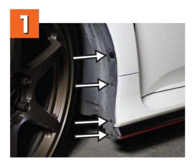
A. Turn your vehicle's front wheels as much as possible to allow access to the fender liner screws/clips.
