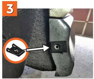
A. Grab one supplied spring u-nut(F) and slightly pry it open to ease installation.
