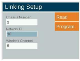
6. Scroll to the Wireless Channel field, select desired Wireless Channel (1–10). The channel will need to be assigned the same to all Wireless Linking Modules installed on-site.
