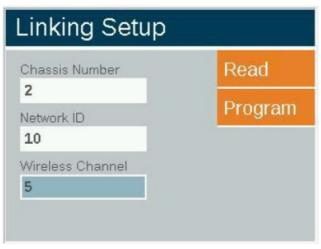
7. Scroll to Program and press the scroll wheel. "Assignment Succeeded" will appear at the bottom of the screen. If the assignment fails, repeat the process.
