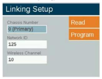
5. Scroll to the Network ID field and select the desired Network ID (0–255). The Network ID will need to be configured the same on all Wireless Linking Modules installed on-site.
