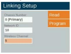
7. Scroll to Program and press the scroll wheel. "Assignment Succeeded" will appear at the bottom of the screen.
