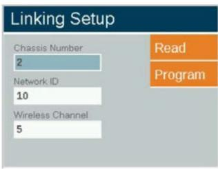
5. Scroll to the Network ID field, select the desired Network ID (0-255). This Network ID will need to be configured the same on all Wireless Linking Modules installed on-site.
