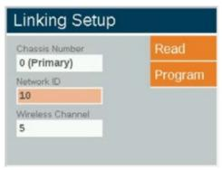
6. Scroll to the Wireless Channel field and select the desired Wireless Channel (1–10). The channel will need to be configured the same on all Wireless Linking Modules installed on-site.
