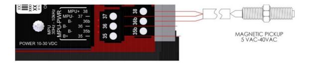
**NOTE:** The MPU input requires a minimum signal of 2 Vrms when connected.
