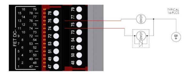
NOTE: If an inductive load does not have an internal flyback diode, it is recommend you install a 1A 600V PIV diode in parallel with the load.
