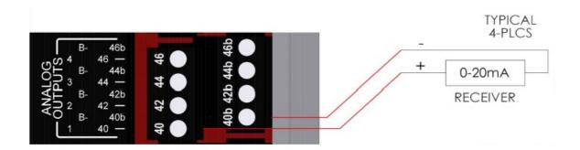
**NOTE:** The MX5-R2 provides all operating power (~B+) to the transmitter and receiver and any other loop components.
