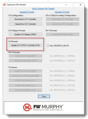
2.7 A new window will appear that allows navigation to the location of the Core CPC4-1 firmware file supplied by FW Murphy. Click OPEN. In the example below, the S19 firmware file is located on the desktop. Double click the S19 file.
