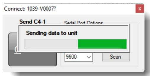
2.10 When the transfer operation is complete, the software will display DONE. Click OK to exit the window and complete the process.
