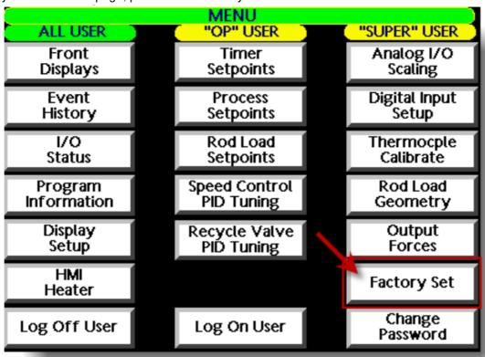
2.13 Next press the Factory Set button on this page. A prompt will appear requiring login using SUPER as the name and the Super user passcode. Refer to the sequence of operation for the panel for proper login credentials. 2.14 After a successful login, follow the display commands to restore the factory settings to the system after a firmware update.
