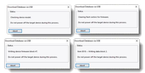
3.12 When the download is complete, the Display will automatically reboot and run the new software. Close the Crimson © software and disconnect the USB cable.
