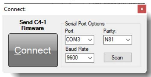
\*If the SCAN button fails to detect the port number, pick the COM port assignment determined by the USB to Serial Bridge manually.
