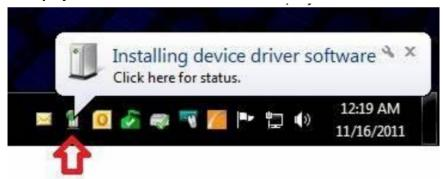
**NOTE:** Please wait until the new hardware is detected and installed, the process can take several minutes. 3.5 After the USB drivers are set up, run Crimson© software by selecting Crimson© from the Windows Start Menu, select Programs and find Red Lion Controls -> CRIMSON X. The version will vary based on what was needed for your Centurion PLUS system. (Windows 10 view similar photo on right.)
