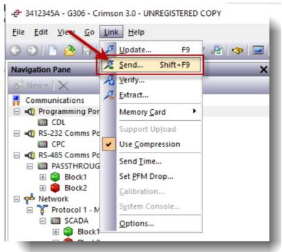
3.11 The transfer to the display will begin. Note this process will also update the firmware in the display if it is not the same as contained in the Crimson© software. Your display may reboot once or twice as new firwmare is loaded prior to the screen database file.
