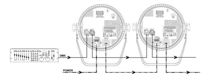
• At the last fixture, the DMX cable has to be terminated. Solder a 120 Ohm resistor between signal (-) and signal (+) into a 3-pin XLR connector and plug this into the DMX output of the last fixture in the chain.
