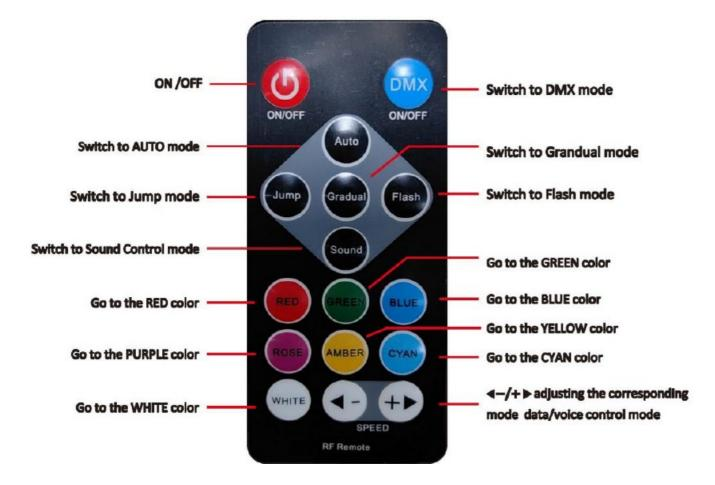
Please note: to use the remote control, you need to first turn on the remote control function of the product. During the use of remote control, please do not use DMX control. During the use of DMX control, please do not use the remote control. Otherwise, signal interference may occur.
