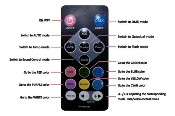
Please note: to use the remote control, you need to first turn on the remote control function of the product. During the use of remote control, please do not use DMX control. During the use of DMX control, please do not use remote control. Otherwise, signal interference may occur.
