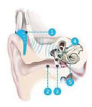
Bone conduction technology creates sound waves by vibrations, sound transmit via temporal bones to your inner ear
