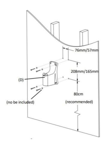
1. Using your electric drill, 3mm (1/8") drill bit, and bubble level, drill the hole Pattern
