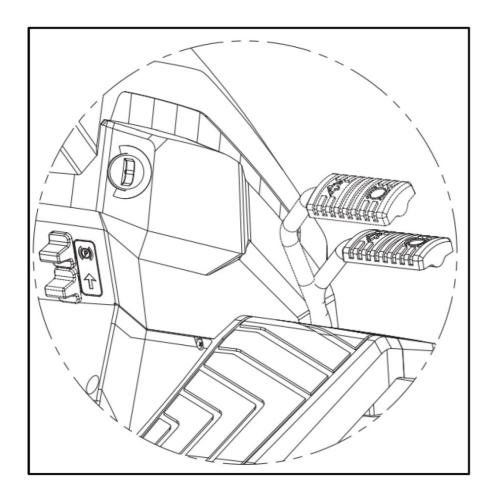
Insert the ignition key and turn it to ON for electrical contact, then turn it to start the engine. Release the ignition key after the engine starts. Once the engine is started, switch throttle control to the minimum speed position.
