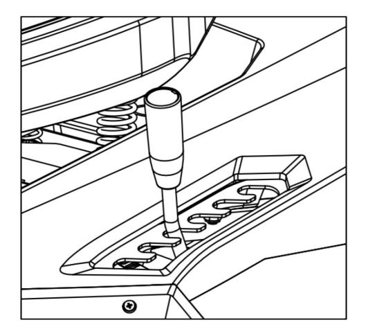
Switch throttle control to the max speed position. Blade clutch at OPEN "B" position.
