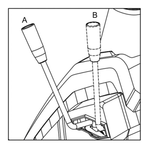
Move the clutch into the starting position
