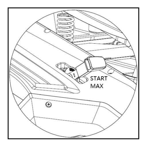
Fully press down the brake pedal and move the gear shift lever to the first position (to control the speed according to adjust to different position), then release the brake pedal slowly.
