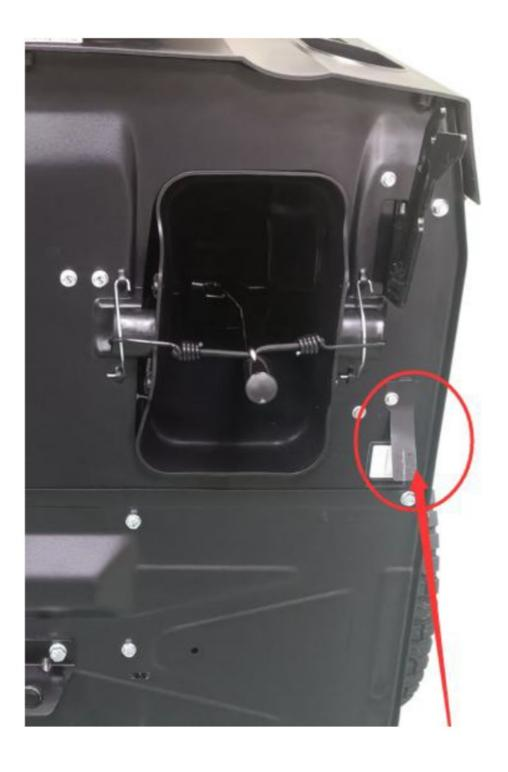
Install the grass catcher on the mower using the hinges provided for this purpose
