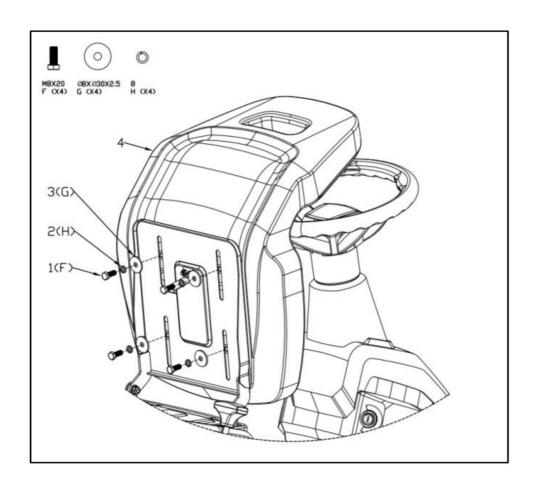
Fasten the seat to the machine using the screw (M8x18) and nut (M8).
