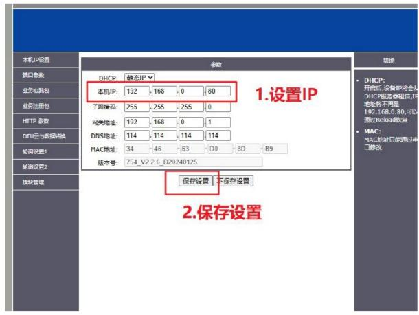
Modify the new IP address, click Save Settings, and restart the module to complete the modification
