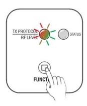
Model WDS-CRMX TX can switch the transmission protocol in TX (transmitter) mode. The setting determines which frequency band is used and if legacy G4 and G3 units can be used in the wireless environment.
