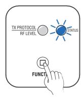
1. Briefly press FUNCTION 5 times. Then press and hold FUNCTION for at least 3 seconds, until the state of the blue LED changes. The unit enters RX/TX selection mode.
