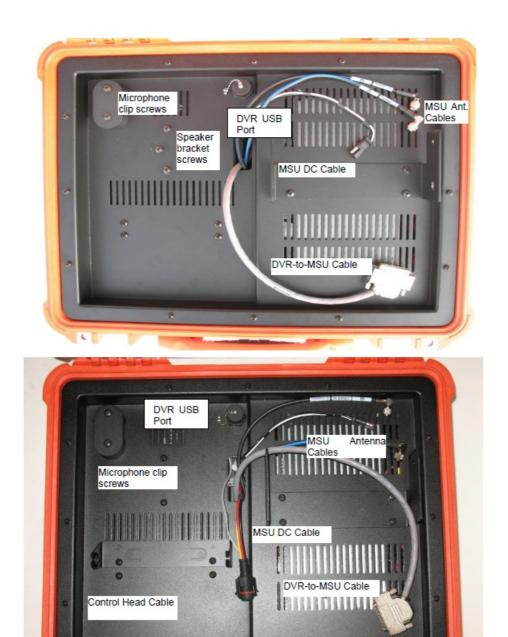
2. STEP 2 Install the microphone clip and speaker bracket as shown on Figure 5, Figure 6 and Figure 7 below. Connect the speaker connector to the CH harness.
