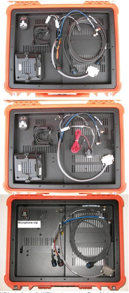
3. STEP 3 Install the MSU using the supplied MSU thumb screws (see Figure 8 below).
