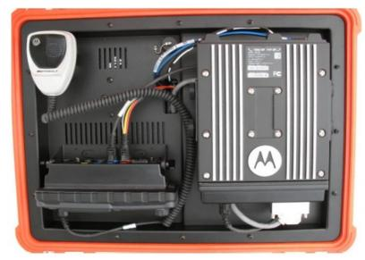
6. STEP 6 Program the MSU, DVR and Portables for DVRS operation. Ensure the templates are fully matched by following the Guidelines provided in the DVRS Programming Guide. To program the DVRS, connect a PC with compatible Tweaker Programming Software to the DVR USB port located under the cap behind the MSU Speaker at the back end of the suitcase.
