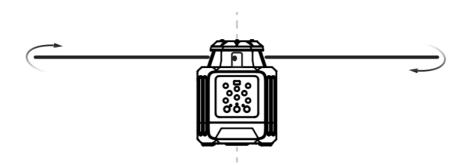
After turning on the device, the laser light blinks without spinning. The laser is levelling. When levelled, the laser beam will light continuously and the laser will start spinning at 600 RPM, the optimal speed for usage with a receiver.
