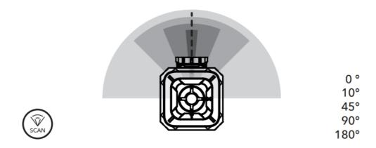
The scan function allows to limit the laser beam to an angle instead of the complete 360° circle. This creates a light intensive segment that increase the visibility for the human eye. Possible angles of the scan function are 0°, 10°,45°, 90° and 180°.
