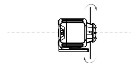
Put the device on its feet vertical mode [10] for vertical alignment (keypad should be on top). The laser will blink without turning during levelling. When levelled, the laser beam will light continuously and the laser will start spinning at 600 rotations per minute, the optimal speed for usage with a receiver.
