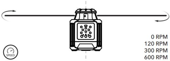
This device has multiple spinning speeds. 0, 120, 300 and 600 RPM (rotations per minute). The default rotation speed is 600 RPM.
