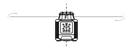
Thanks to the plumb lines, which are projected via Plumb point up [02] and Plumb point down [08], this device can also be used to bring a plumb lead point of the fl oor to the ceiling, or vice versa.
