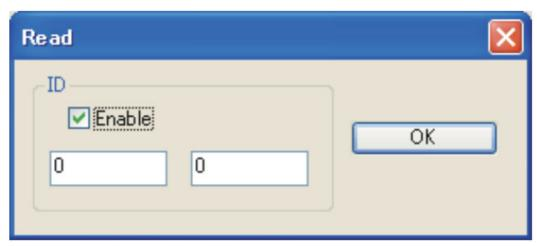
\* When only one servo is connected to the CIU-2, after deselecting by checking the "Enable" check box; press the "OK" button. The parameters are read.
