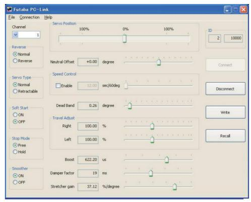
\* When reading of the parameters failed, an error message is displayed. In this case, recheck the connection and ID and read the parameters again.
