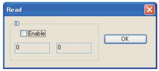
\* When multiple servos are connected to the CIU-2, confirm that the "Enable" check box is checked and enter the ID given on the servo whose parameters you want to read and press the "OK" button. The parameters are read. (The gure below shows the case when the servo ID is "002-10000".)
