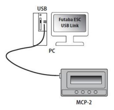
Sometimes the firmware of Program box should be updated because the functions of ESC are improved continuously. Connect the Program box with PC through USB port, run Hobbywing USB Link Software, select "Device" "Multifunction LCD Program Box", at the "Firmware Upgrade" module, choose the new firmware you want to use, and then click "Upgrade" button.
