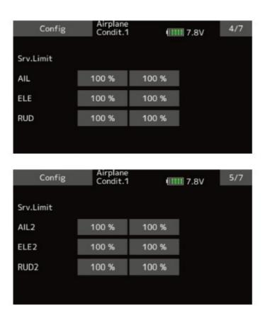
This is the limit setting for each servo. The position of the maximum operation is read into the gyro in the first setting.
