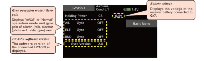
On the home screen, basic information such as gyro operation mode, sensitivity, battery voltage are displayed.
