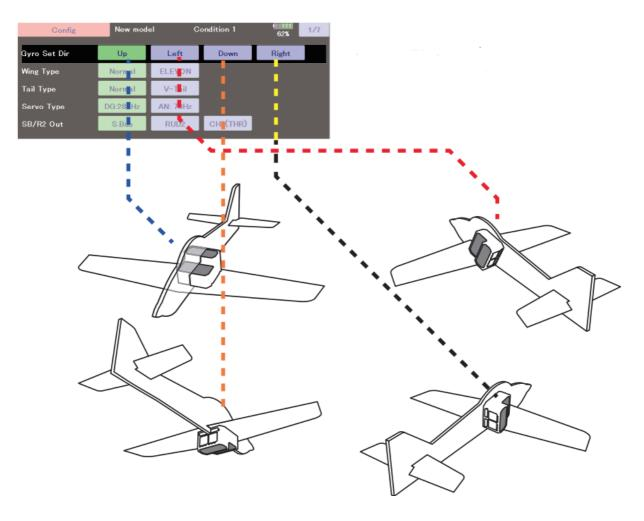
Set the mounting direction of GYA. Set mounting direction
