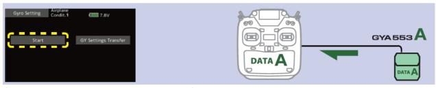
• Connect the gyro A to the T32MZ and press [Start]. (Enter the data of A into T32MZ)
