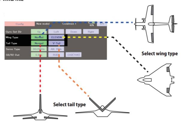
Set with the wing type/tail type of GYA553. The wing type/tail type of the transmitter is not used and is normal.
