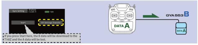
• Connect Gyro B to T32MZ and press [GY Settings Transfer]. (Put data on A into gyro B)
