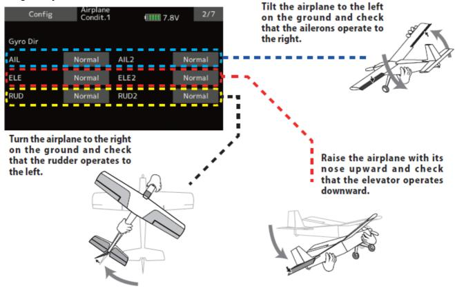
It is the direction settting of the gyro. Be careful as it will crash if the direction is reversed. For dual aileron, dual elevator, and dual rudder aircraft, check the operating direction of each second aileron/elevator/rudder.
