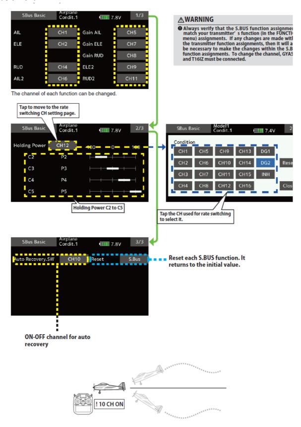
Set the CH for each function according to the transmitter to be used. Any unused functions should be set to INH (Inhibited). The channel of each function can be changed.
