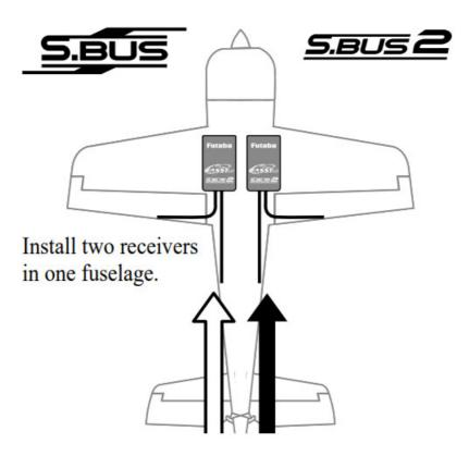
**FDLS-1** is a secure system. In the event of trouble with the main receiver, the **FDLS-1** will automatically switch to the sub receiver and fly safely
