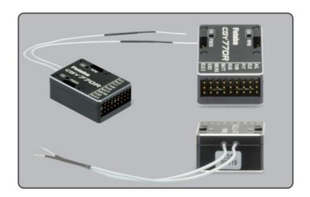
Futaba CGY770R is gyro, 3-axis Stabilization System combining AVCS gyro and head speed governor and receiver in one box designed for flybarless helicopters. Its cutting-edge MEMS (Micro Electro Mechanical System) sensor design, ultra high-speed processing speed, and advanced PID control algorithm put it a league of it's own
