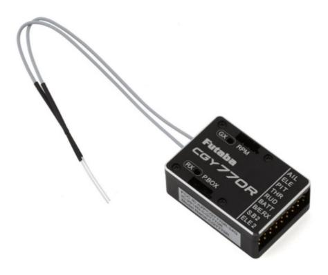
3-axis AVCS Gyro Gyro/Receiver/Governor function integrated Compatible with flybarless helicopters
